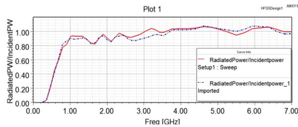
Fig. 5. The Radiated Power / Incident Power vs. Frequency
