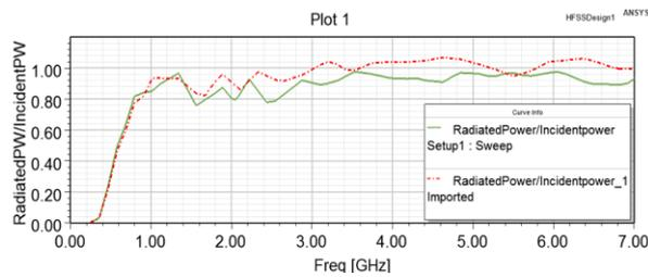
Fig. 15. The Radiated Power / Incident Power vs. Frequency
