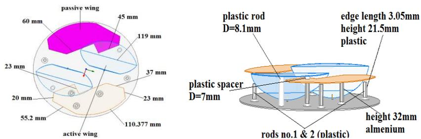
Fig. 1. MIMO 2×2 antenna Circular shape
