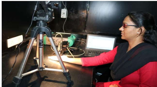
Fig. 7. Laboratory Experimental Measurement Setup of Palmprint Spectra
